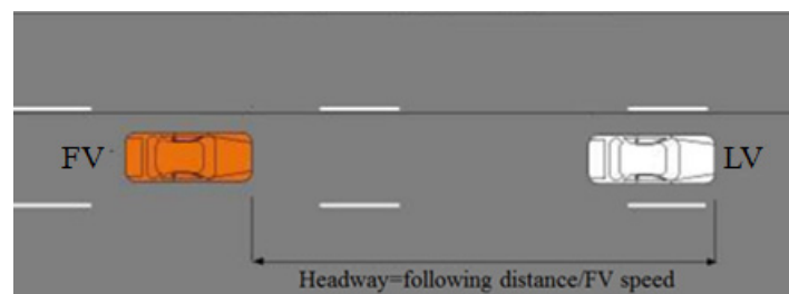
Figure 3. Calculation of vehicle headway.
